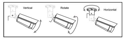
Step 3: Power on the camera and fine-tune the viewing angle. Please go to the section, "ADJUST FOCAL LENGTH & FOCUS", for details.
